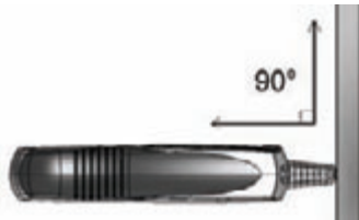
Figure 4-1 Correct measuring angle
